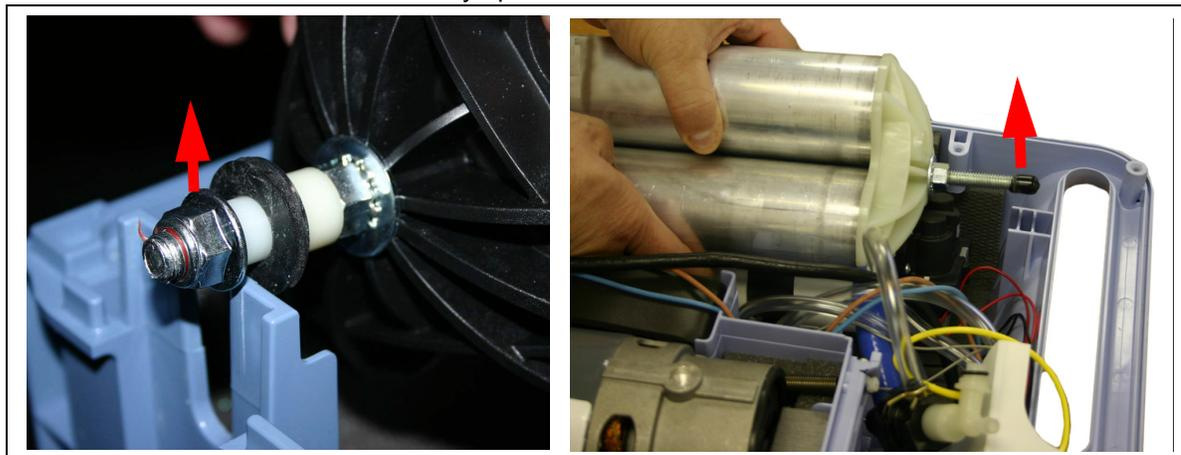
**FIGURE 8-17: SIEVE CANISTER ASSEMBLY REMOVAL**
