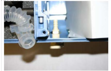
23. Thread the locking nut to the O2 Quick Coupler and tighten.
