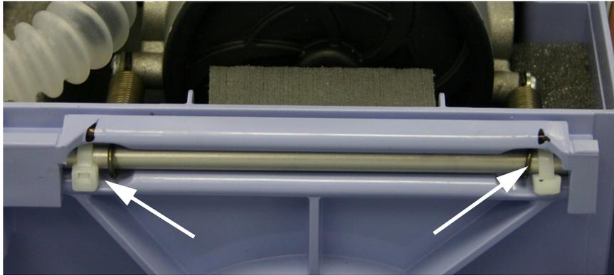
**FIGURE 8-22: MOUNTING ROD TIE WRAPS**
