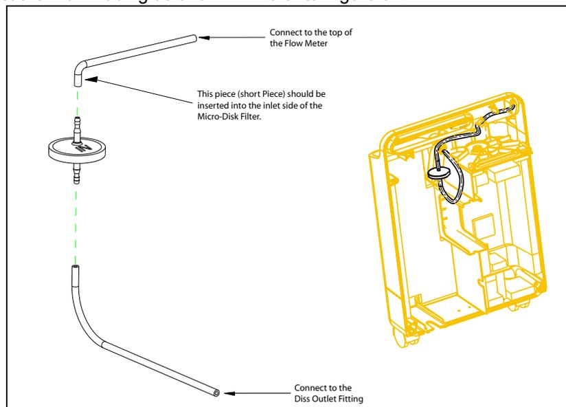
**FIGURE 8-27: FLOW TUBING INSTALLATION**
