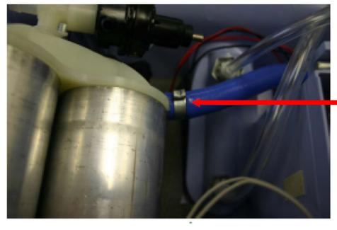
10. Remove the Sieve Canister Assembly from the Front Cabinet.
