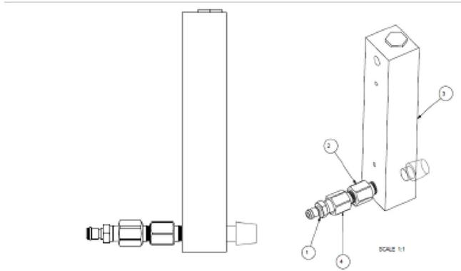
**FIGURE 10-1: TEST FLOWMETER ASSEMBLY**
