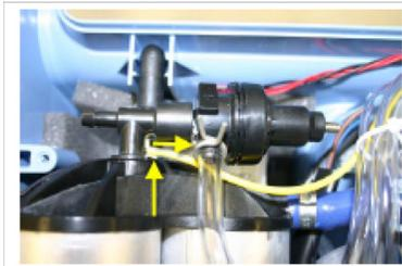
7. Remove the Pressure Regulator Assembly from the Sieve Assembly by rotating the Regulator Assembly "up" and pulling away from the Sieve Assembly as shown below.
