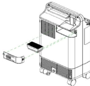
3. Remove the (4) 5/16" Hex screws and (2) Phillips head screws as shown below.
