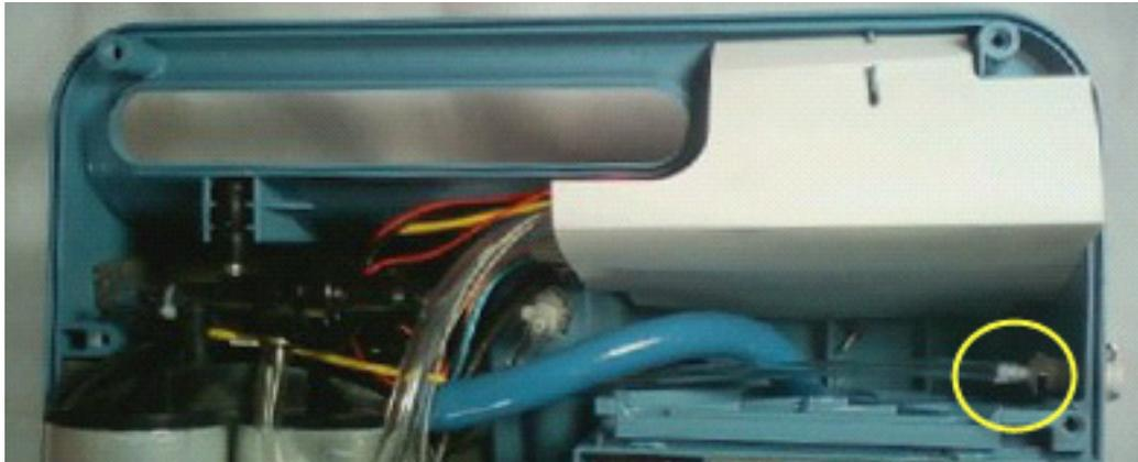
5. Remove the securing nut from the coupler and push the coupler towards the outside of the device to remove.
