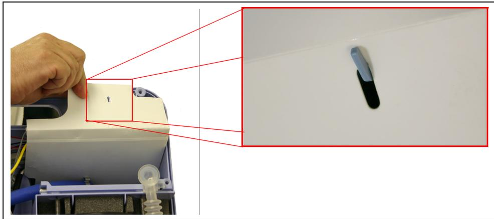
**FIGURE 8-7: UNCLIP MAIN PCA**
