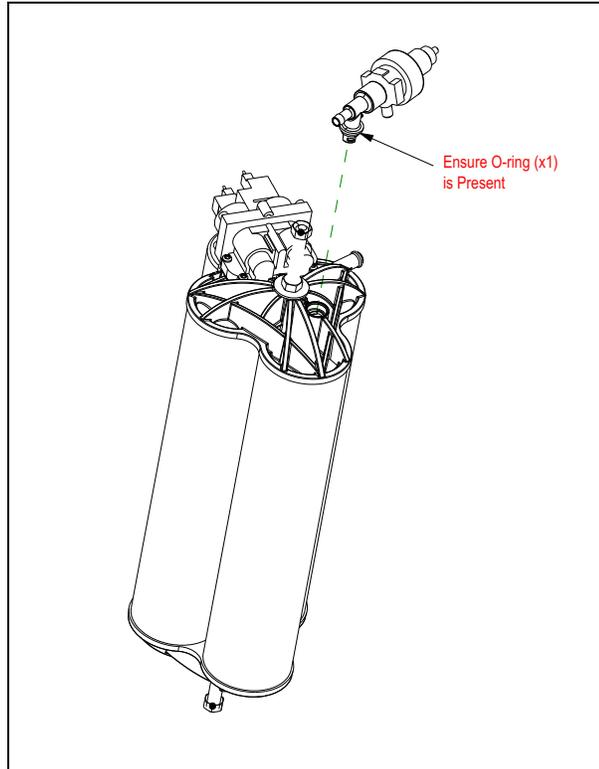
**FIGURE 8-10: PRESSURE REGULATOR ASSEMBLY REMOVAL/INSTALLATION**
