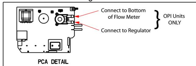
**FIGURE 8-26: PRESSURE TUBING CONNECTIONS**
