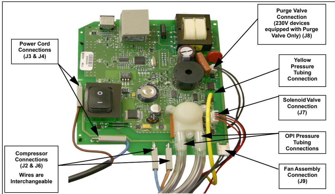
**FIGURE 8-15: CONNECTION POINTS ON THE MAIN PCA**
