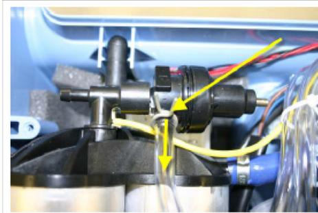
6. Remove the yellow tube from the Pressure Regulator as shown below.
