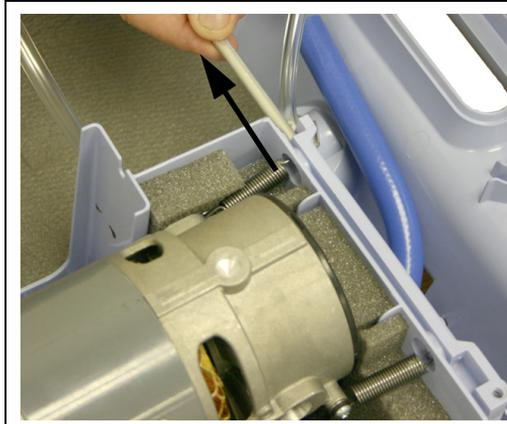
**FIGURE 8-23: MOUNTING ROD REMOVAL**
