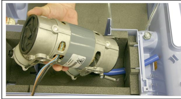
**FIGURE 8-24: COMPRESSOR REMOVAL**
