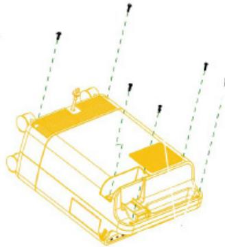
26. Replace the Long Life Filter and Filter Cover as shown below.
