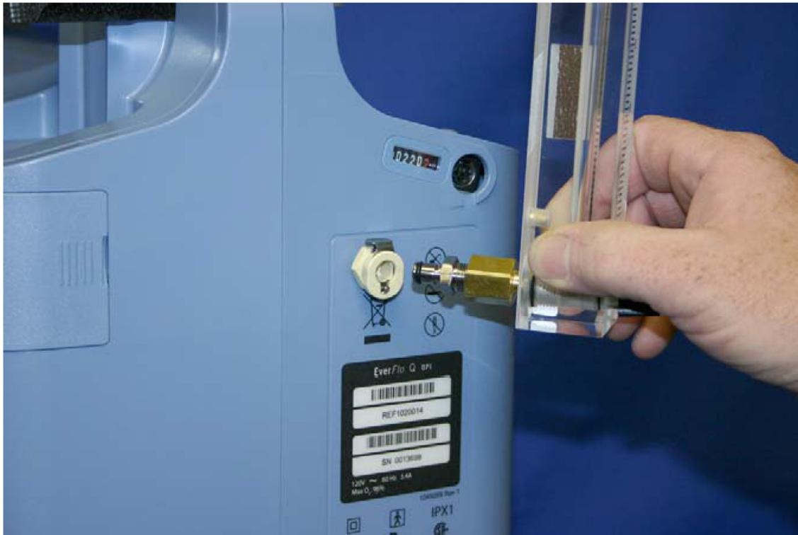
12. Open the Test Flowmeter flow knob 3-4 turns.
