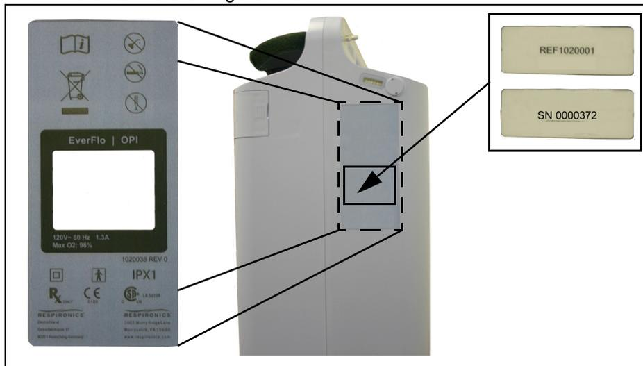
**FIGURE 8-30: NEW SERIAL/MODEL NUMBER LABEL PLACEMENT**
