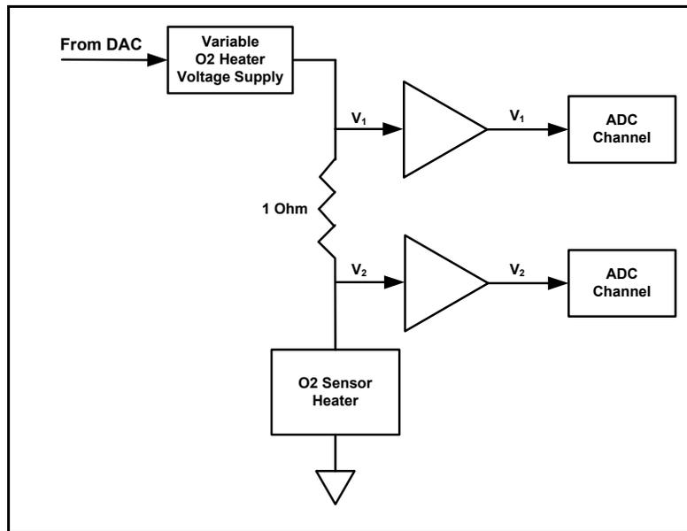
As can be seen from the above quasi-schematic, the instantaneous power being delivered to the heater element of the O<sub>2</sub> sensor is equal to,
