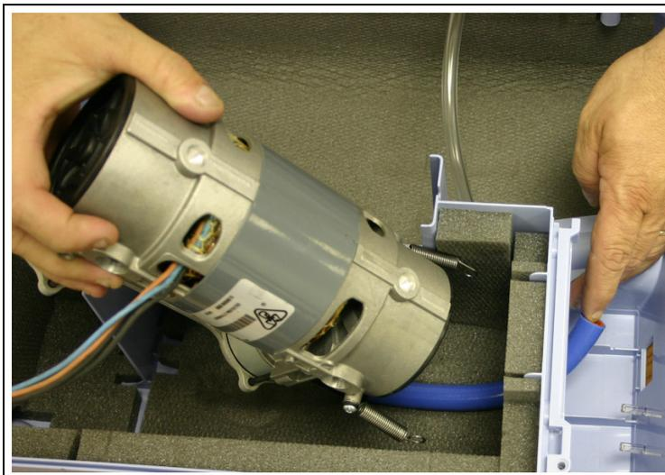
**FIGURE 8-25: COMPRESSOR PLACEMENT INTO FRONT CABINET**
