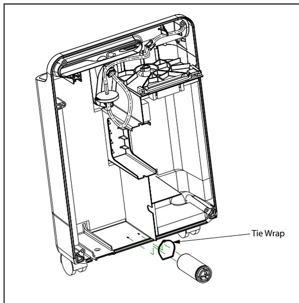
**FIGURE 8-21: CAPACITOR REMOVAL/INSTALLATION**
