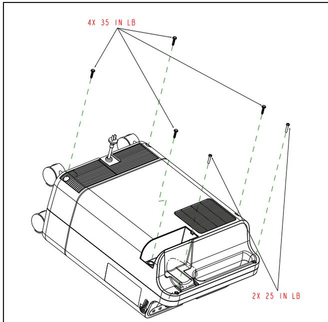
**FIGURE 8-3: SCREW REMOVAL/INSTALLATION**
