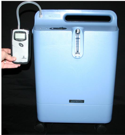
3. Set the flow to 5 lpm (1 lpm for units equipped with pediatric flow meters).
