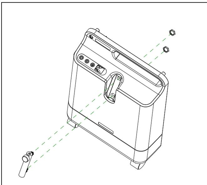
**FIGURE 8-28: FLOW METER REMOVAL/INSTALLATION**
