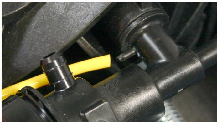
**FIGURE 8-11: PRESSURE LINE REMOVAL**
