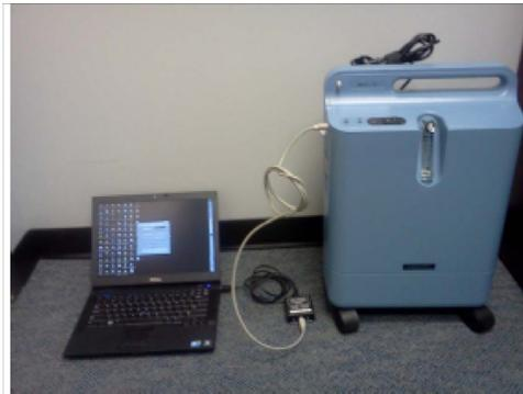
37. Run the software to install the correct firmware into the device. Once complete disconnect the COM Box from the EverFlo Device and proceed to the testing section of the service manual.
