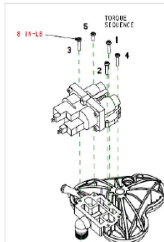
13. Install the EverFlo upgraded for use with UltraFill Pressure Regulator to the top of the Sieve Assembly.
