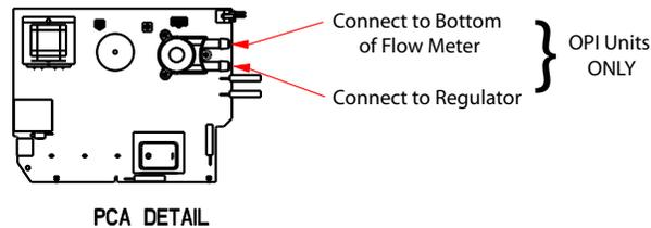
3. Connect the Valve Solenoid connector to the J7 location of the Main PCA. Refer to Figure 8-15.
