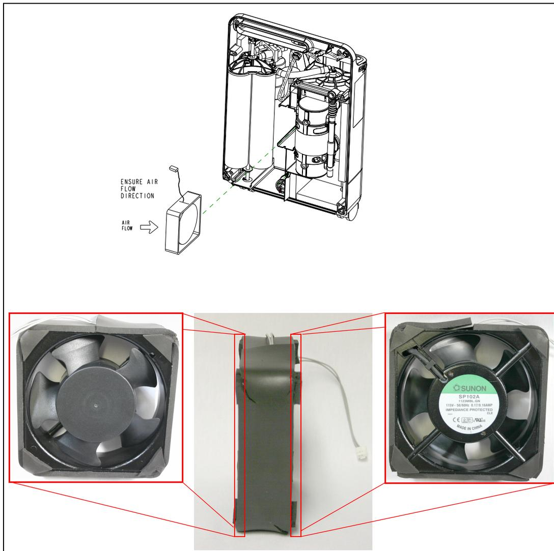
**FIGURE 8-20: FAN REMOVAL/INSTALLATION AND PROPER ORIENTATION**
