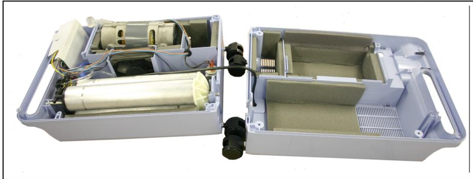
**FIGURE 8-5: EVERFLO REPAIR POSITION**
